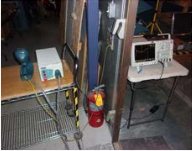
CS118 Verification, Current
