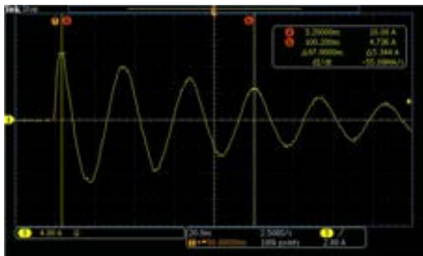
CS116 Generator Calibration: 30MHz
