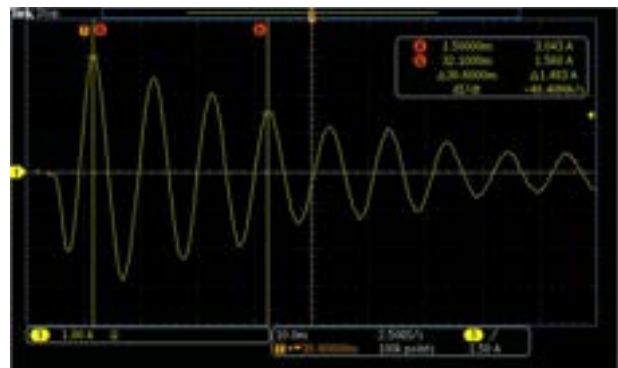
CS116 Generator Calibration: 100MHz
