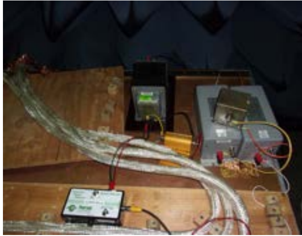
CS101 Calibration Setup (Alternate View)
