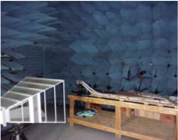
RE102, 200MHz-1GHz Vertical Position 1
