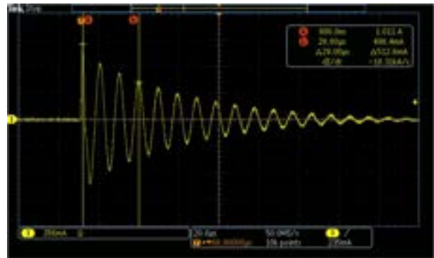
CS116 Generator Calibration: 100kHz
