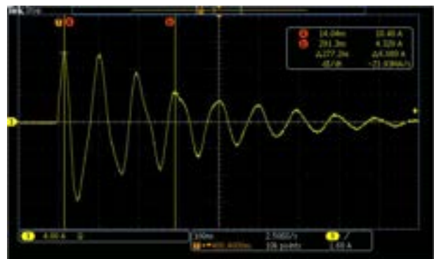
CS116 Generator Calibration: 10MHz
