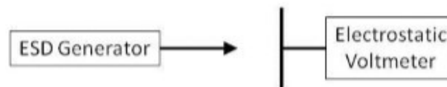
Figure 5.6-1: Measurement System Check Setup, Tip Voltage Verification
