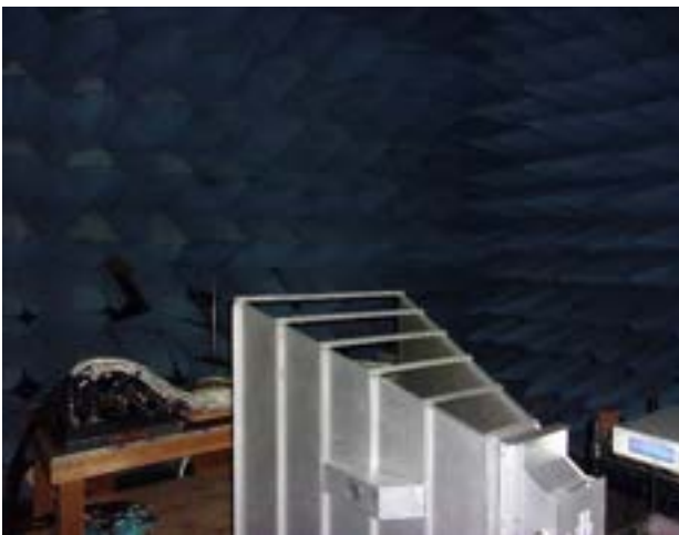
200MHz-1GHz Stub Radiator
