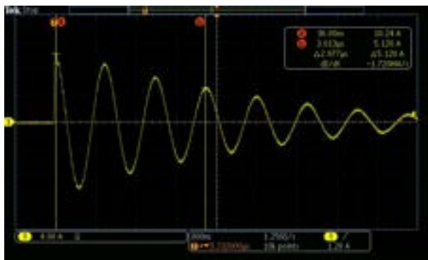
CS116 Generator Calibration: 1MHz
