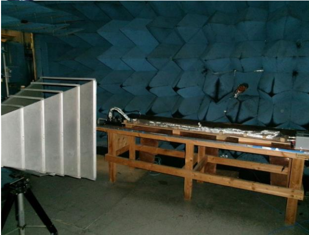
RE102 Test, 200MHz-1GHz, Horizontal, Position 1
